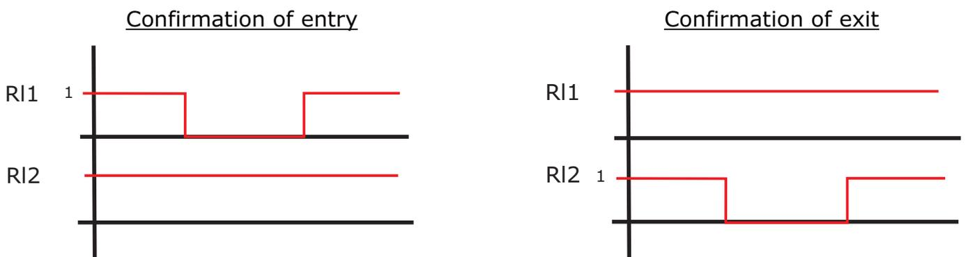
In this operation mode, the output RI1 can be used to activate an electromechanical counter in order to count the passage flow in the direction of entry of the equipment. Similarly, the output RI2 can be used to count the passage flow in the direction of exit.
