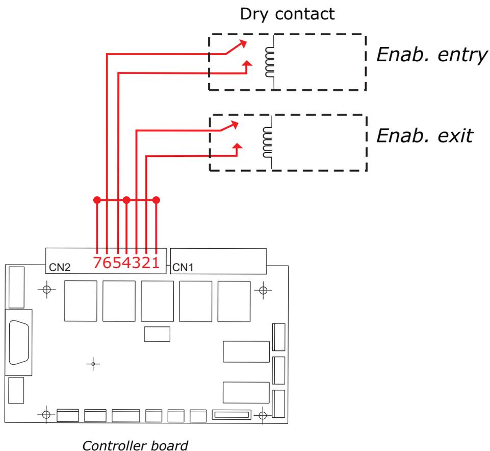
**Enabling by solid state (positive, positive voltage):**
