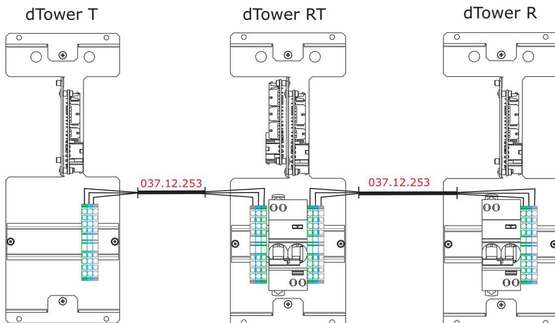
**NOTE** - On the cable itself there are rings identifying where each cable must be connected.
