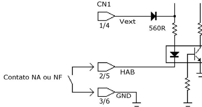
Enabling passage through tension pulse is shown in the image below. It is necessary to observe the polarity of the Vcc voltages and to use an external resistor for high voltages (110V and 220V).
