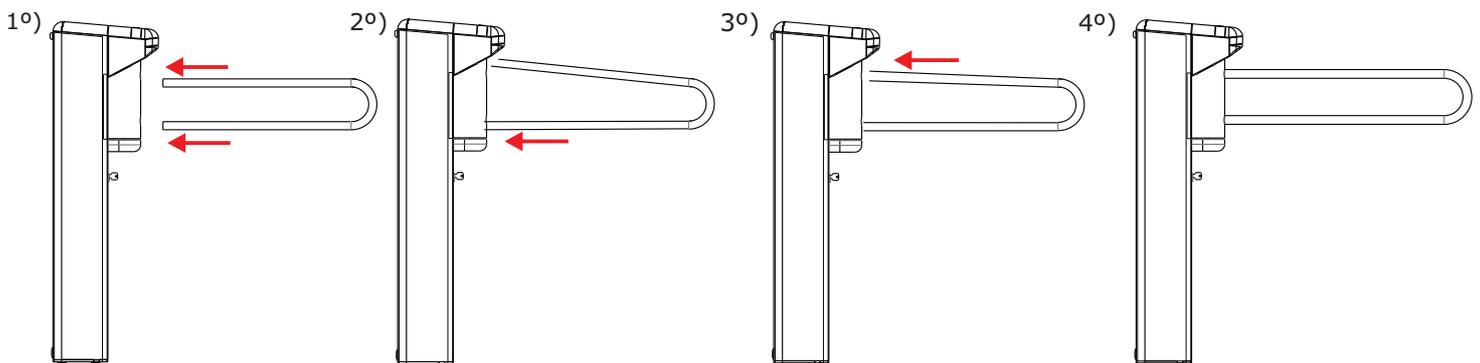
2. Once the arm has both rods duly fitted, turn the arm to one side up to about 180 degrees or until it reaches the end of its track. You will notice there are two holes on the back of the tube.
